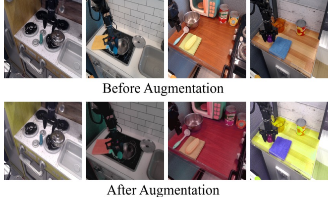
Fig. 4: Image augmentation examples Examples of images from the Bridge dataset before and after having the image augmentations applied to them that are used during policy and classifier training.
